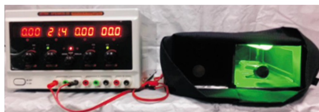
Figure 1 A homemade monochromatic light cell incubator The homemade cell culture incubator was used for culturing rat Müller cells in vitro and treating them with 530 nm monochromatic light. The cell incubator was placed into a normal cell incubator.
