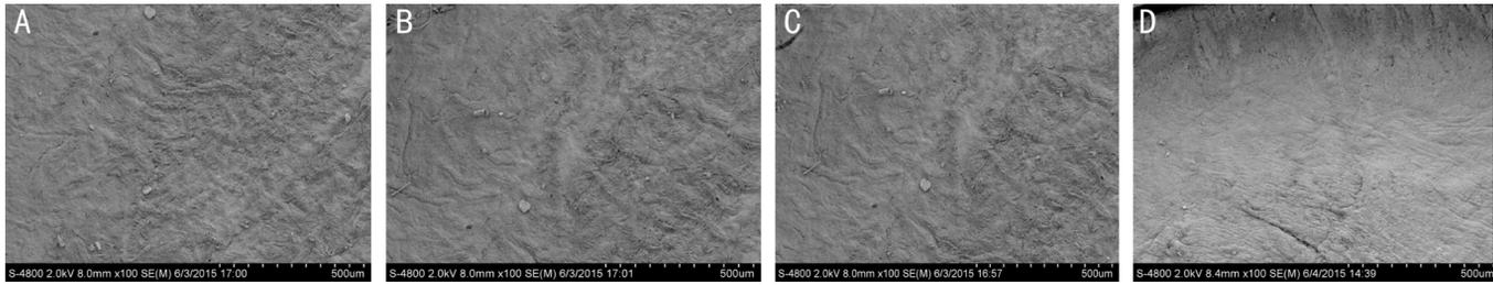
**Figure 4** SEM images at  $\times 100$  magnification were used to evaluate microscopic roughness. Group A showed the worst smoothness. Group D showed the best smoothness. The microscopic roughness in Group B or Group C was moderate level.
