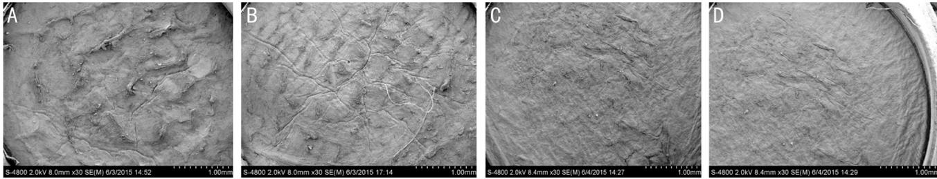
**Figure 3** SEM images at  $\times 30$  magnification were used to evaluate the severity of the ridges. Group A showed the maximum ridges. Group D showed the minimal ridges. The ridges in Group B or Group C was intermediate level compared to the other groups.
