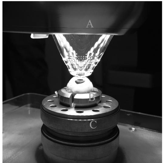
applanation cone (A). At the top of holder, four arms (B) hold the eyeball to make its proper position and pressure. As the rotation of top rounding screw (C) of the the holder, the strength of arm of the holder will be adjusted in order to control the pressure of the eye ball.
